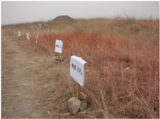
图1 连续喷洒不同浓度的阻燃剂 Fig.1 Continuous spraying at different flame retardant densities
