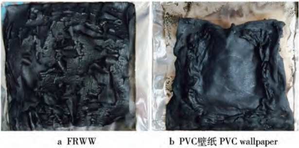
图3 燃烧后的阻燃木质壁纸、PVC 壁纸残炭 Fig.3 Carbon residues of FRWW and PVC wallpaper after burning
